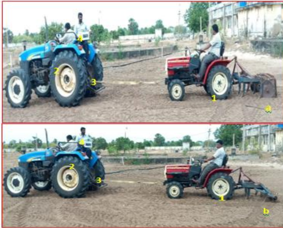
Fig. 5. Draft force measurement of developed combination tillage implements 1. Test tractor with implement; 2. Auxiliary tractor; 3. Load cell; 4. Digital indicator; a. cultivator-disc harrow; b. cultivator-clod crusher
