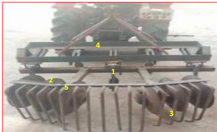
Fig. 1. Developed passive-passive combination tillage implements C-DH with test tractor 1. Supporting frame; 2. Disc harrows; 3. Weed collector; 4. Front passive set; 5. Rear passive set
