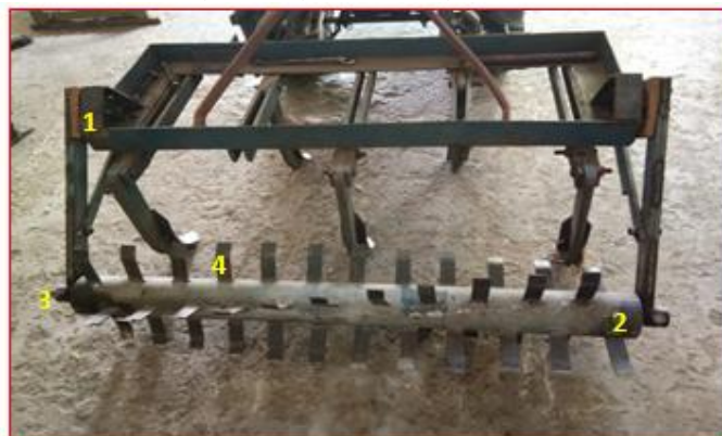
Fig. 3. Schematic diagram of cultivator with clod crusher 1. Frame; 2. Arms ; 3. Cultivator; 4. Clod crusher
